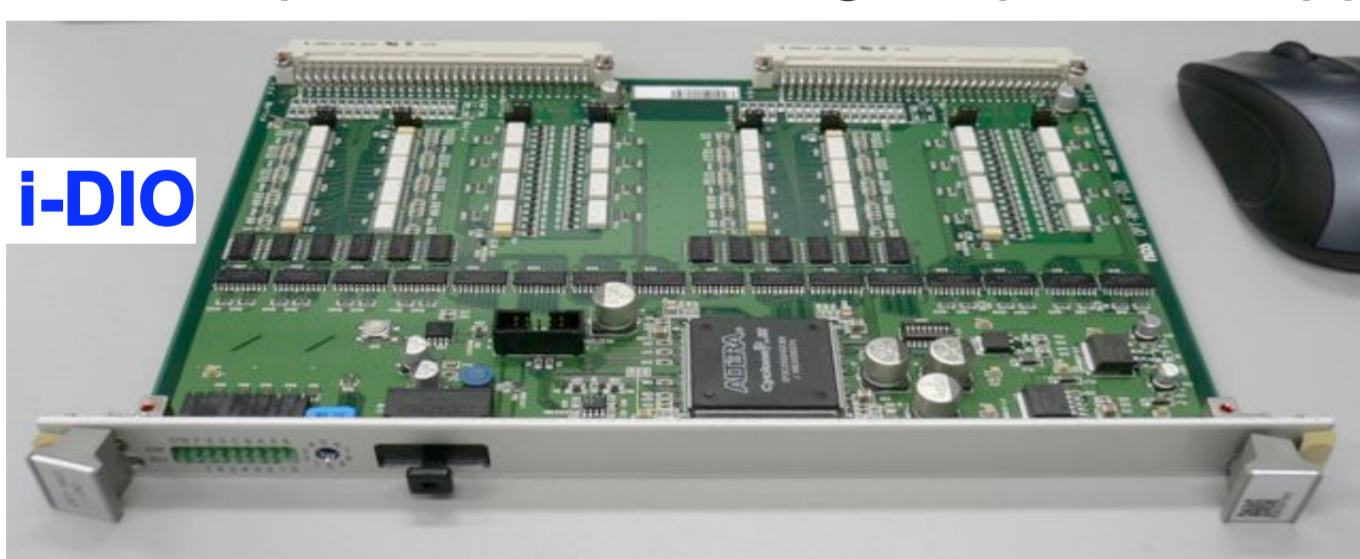
The i-DIO is inserted into the PS rear panel.
