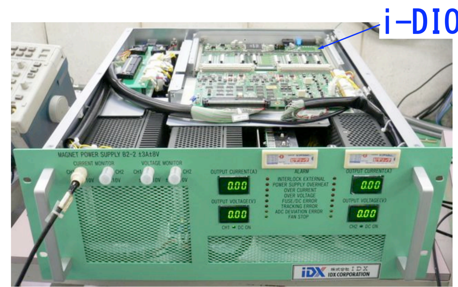
Front and top view of 2ch magnet power supply
