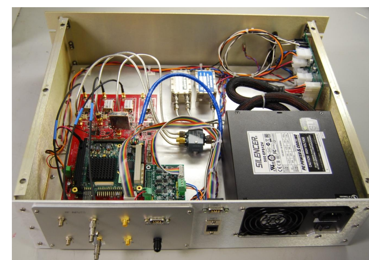
Diagnostic Receiver (custom FPGA-based PCB)
