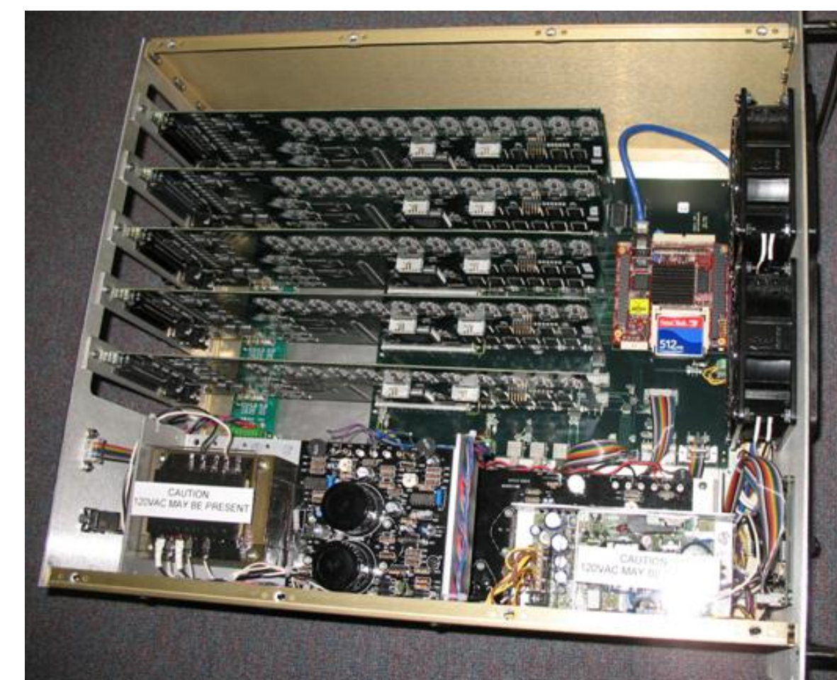
Distributed Data Acquisition (custom FPGA-based PCB)
