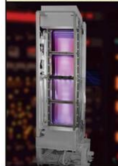
Plasma Electrode Pockels Cell (192)
