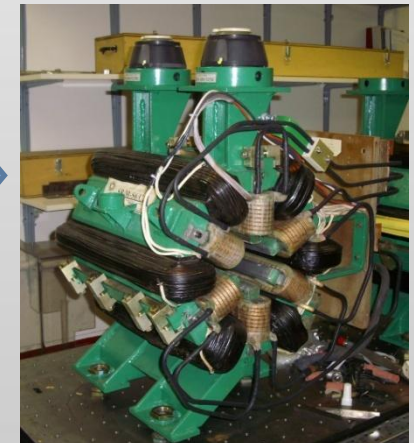
The correctors are part of the sextupoles (6 black coils)
